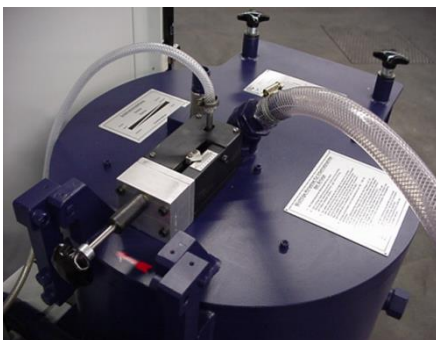
Three phase separator SMR 100 - the core of the system
