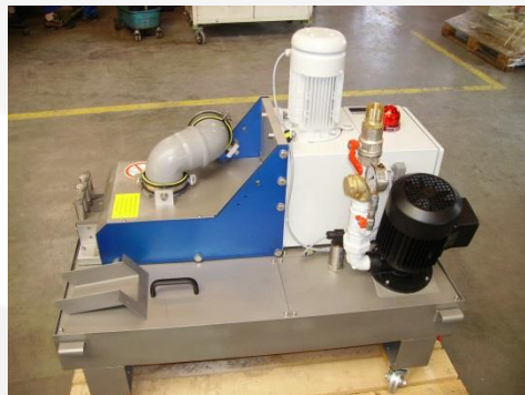
KP 60 - B 150 Plastic material press with collecting tank
